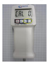
**3.** Wait a few seconds and display will show the necessary adjustment weight, e.g. 5,000kg for FK 50 or 10,00kg for FK 100.
