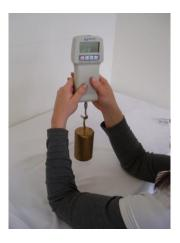
5. Hold position until "F" appears on display. In this case remove weight and adjusting is completed. In case of "E" showing up on display - repeat step 1. to 5. until "F" attests a successful adjustment
